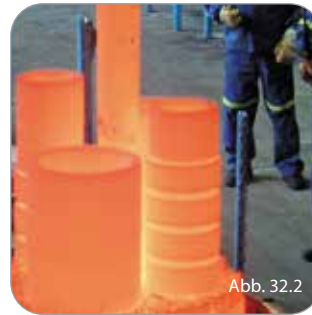
Vergüten, glühende Charge / tempering, red-hot batch
